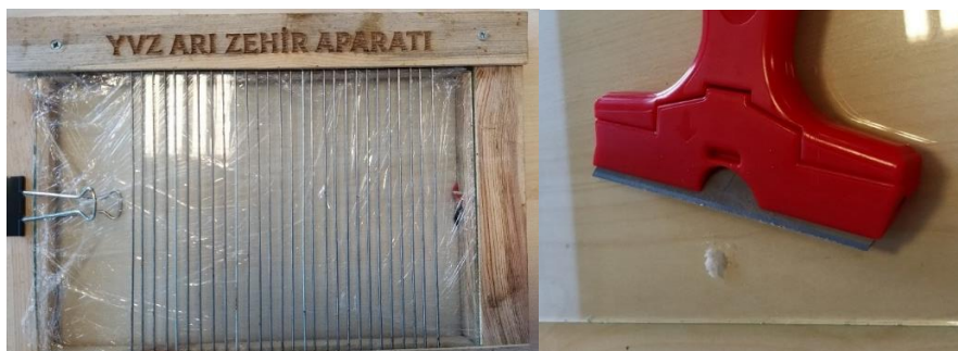
Figure 2: Apparatus for the collection of bee venom
