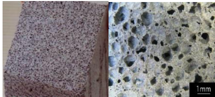
Figure 6. Porous structure of AAC
