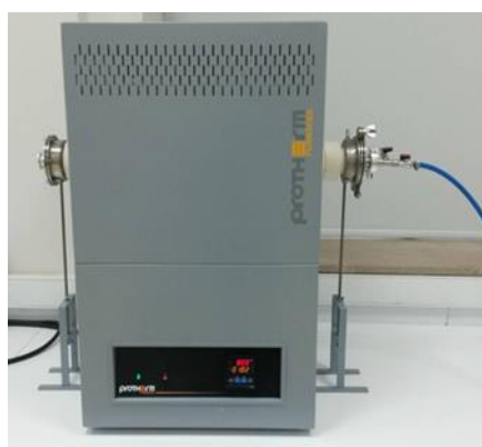
Figure 3. Protherm brand atmosphere controlled heat treatment furnace.
